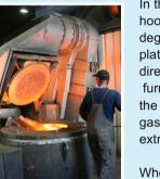
In the filling position, when the hood is positioned in a 60 degrees angle to the furnace platform, the rear opening is directly situated over the furnace. Consequently the thermal of the mounting gases additionally improves the extraction performance.
