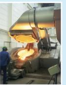
The result is definitely better than with side extraction. When the hood is open, the highest extraction performance is on the rear opening.
